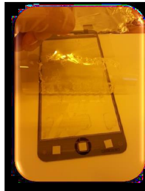
OCA 移除 • 50 \mu m PET Film Backing
